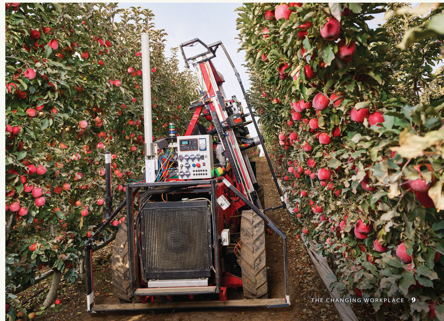
▼ A driverless harvesting robot uses suction to pick apples from trees in Washington State, U.S.A.
